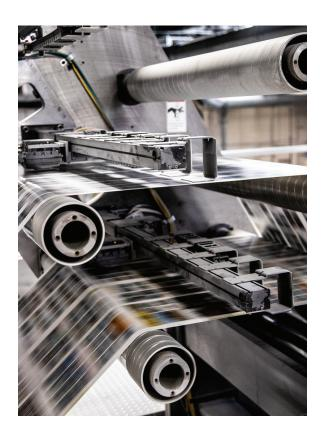
The press facility operates around the clock, leveraging digital, direct-to-plate technology capable of producing 1.76 million pages per hour alongside a bindery capable of outputting up to 22,000 stitched books per hour.
