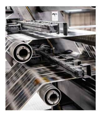
The press facility operates 24/7, utilizing digital direct-to-plate technology to produce up to 1.76 million pages per hour, with a bindery that can stitch up to 22,000 books per hour.
